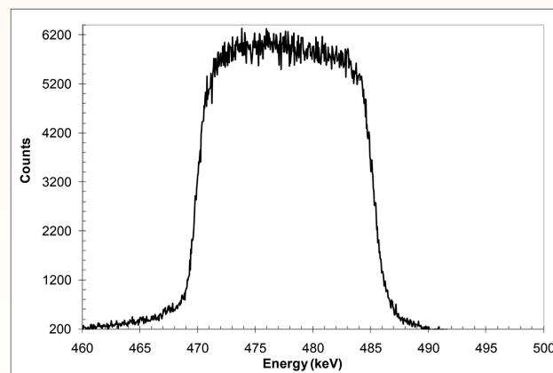
Fig. 3. Counts versus energy for 477 keV gamma-ray measured with an HPGe for slow neutrons incident on BF<sub>3</sub> gas showing the Doppler broadening effect.
