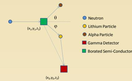
Fig. 4. Geometric layout of the <sup>10</sup>B (n,α) reaction used in the derivation of the incident neutron angle from correlated neutron and gamma detector measurements.
