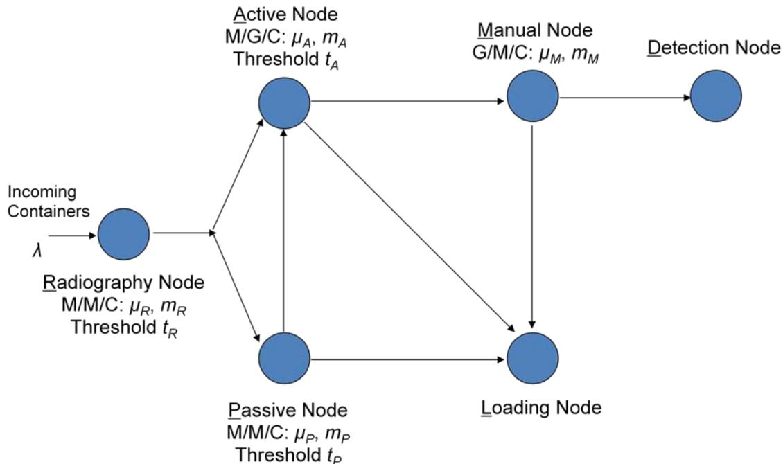
**Figure 1.** Single Port Scenario Port model. Each node indicates a station through which the container must travel in order to be cleared for commerce.
